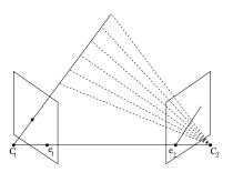
Uncalibrated Structure from Motion with 2 cameras:
