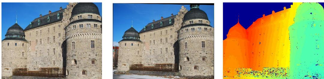
Figure 1: Left and Middle: Two images used for computing depth estimates for every pixel in the left image. Right: The depth estimate color coded.
