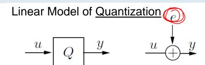
e: Noise independent of u with rectangular distribution over the quantization size with rectangular distribution with variance
