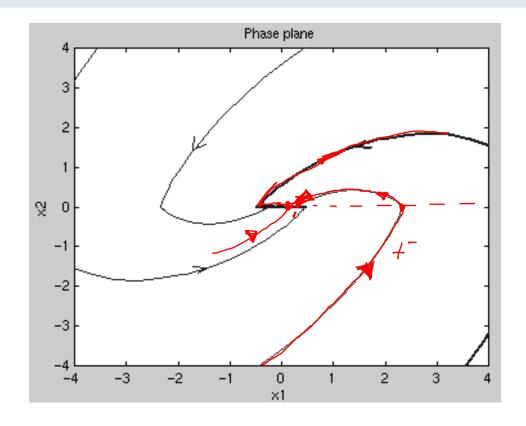
The dynamics along the sliding set in  $\sigma(x)=0$  can also be obtained by finding  $u=u_{\text{eq}}\in[-1,1]$  such that  $\dot{\sigma}(x)=0$ .  $u_{\text{eq}}$  is called the **equivalent control**.
