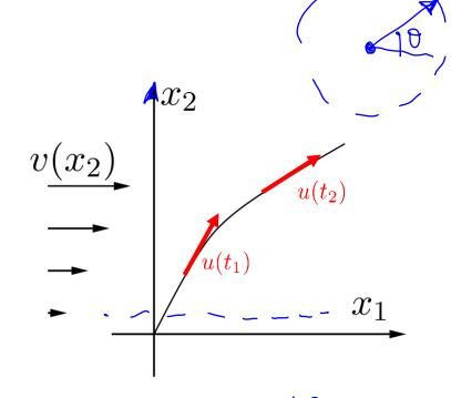
$$\min_{\substack{u : [0, t_f) \to U \\ \dot{x}_1 = (v(x_2)) + u_1 \\ \dot{x}_2 = u_2} + u_1$$
