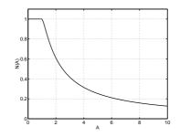
Figure 5.6 Normalized describing function.
