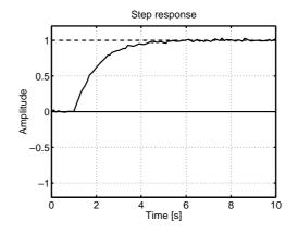
**Figure 7.3** Experimental step response for q = 1.
