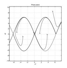
Figure 7.16 Phase plane for pendulum under energy control.
