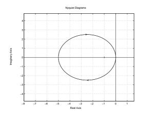
**Figure 7.12** Nyquist curve and -1/N(A) for oscillator example.
