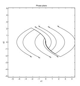
Figure 7.19 Phase plane with switching curve
