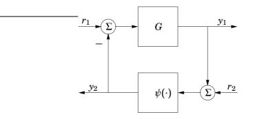
Figure 4.1 Feedback connection form
