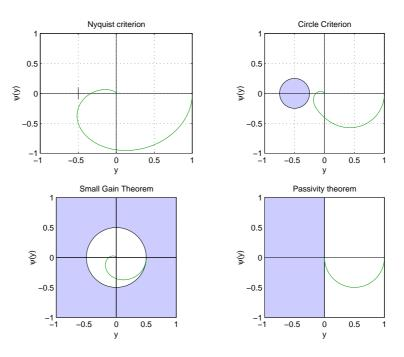
Figure 7.8 Conditions on Nyquist curve matched to sector conditions on memoryless nonlinearity.
