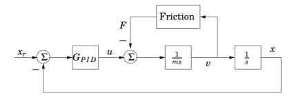
Figure 1.5 Control system with friction in Example 1.6.
