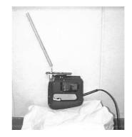
Figure 1.11 The inverted pendulum on an electric hand-saw in Exercise 1.16
