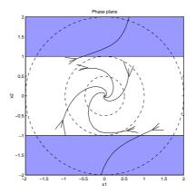
**Figure 7.5** Trajectories of the nonlinear system and level surfaces of  $V(x) = 0.5x^T x$ . The region of attraction is the unit circle.
