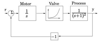
Figure 1.7 Block diagram of system in Exercise 1.8.
