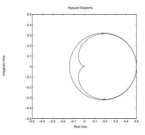
Figure 7.9 The Nyquist curves for the system in Exercise 4.6a, and the circle corresponding to  $k_1 = -2, k_2 = 7$ .
