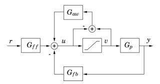
Figure 1.6 Anti-windup compensation in Example 1.7.
