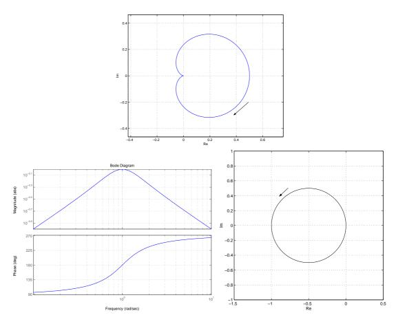
**Figure 4.5** Nyquist curves for the system in Exercise 4.6a (above) and Bode and Nyquist curve for the system in Exercise 4.6b (below)
