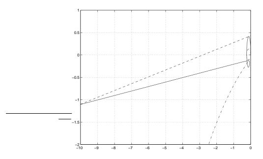
**Figure 4.8** Nyquist (dash-dot) and Popov curve (solid) for the system in Exercise 4.13d. The Popov curve is to the right of the dashed line for all  $\omega$ .
