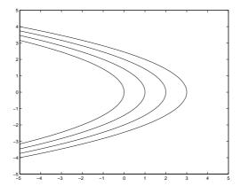
**Figure 7.18** Phase plane for u = -1. The solution is traveling downwards.
