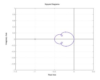
Figure 7.11 Nyquist curve of linear subsystem.
