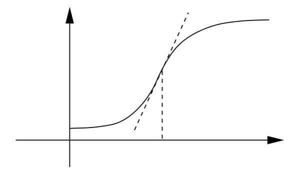
Model of an edge: *Maximum of derivative = position of edge* Two dimensions: Use discrete approximation of
